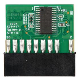
Hardware-based security solution for data protection and reliable authentication via TPM that stores key, passwords and digital certificates.
