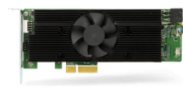
IEI Mustang-V100-MX8 Accelerator with 8 Intel® Movidius™ Myriad™ X MA2485 VPU's
